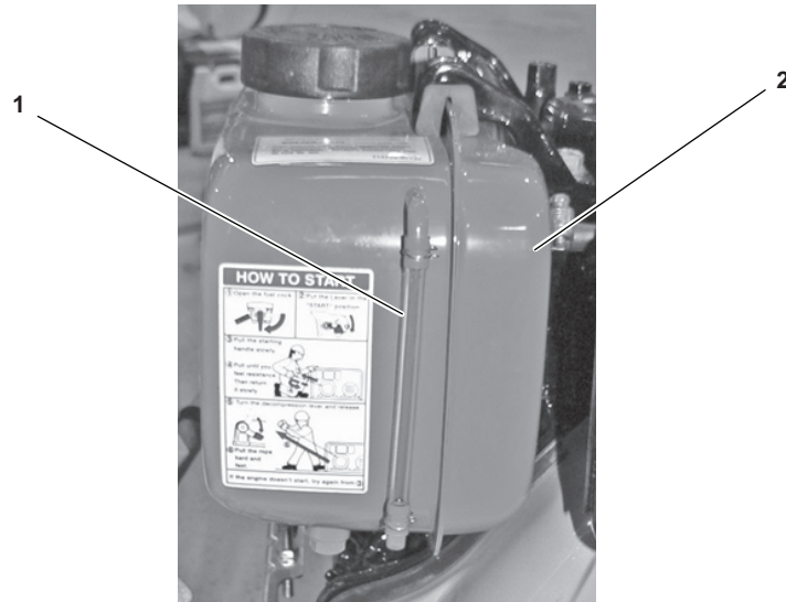
Figure 2-14. Fuel Tank Sight Glass
