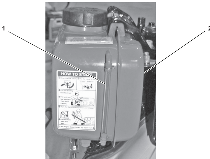
Figure 2-7. Fuel Tank Sight Glass
